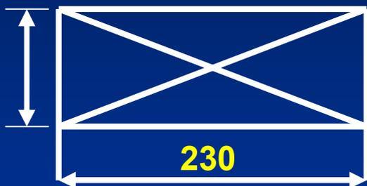
$$\begin{array}{r} 230 \\ \hline 30.48 \times 250 = 1866 \text{ CFM} \\ 1866 \div 35.32 = 53.4 \text{ CMM} \end{array}$$
